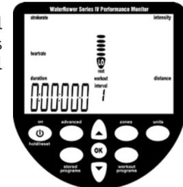
Once the first workout rest duration is reached press “OK” (the duration digits will appear along with the “duration” flag, the “workout”, “interval” and “work” flags will be flashing and the zone bar will be scrolling up to HI. The number 2 will appear in the program window denominating the 2nd work session).
