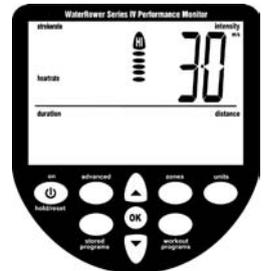
Once the desired upper limit is reached press “OK” (the lower intensity unit digits will appear along with the “intensity” flag and the zone bar will flash scrolling down to LO).
