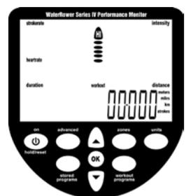
Scroll to the desired workout distance using the arrow buttons. Once the desired workout distance is reached press "OK" and the monitor will return to ready mode. The S4 Monitor's AutoPreview feature will automatically scroll through the distance workout settings.
