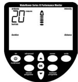
Scroll to the desired intensity lower limit using the arrow buttons. Once the desired lower limit is reached press “OK” and the monitor will return to ready mode.
