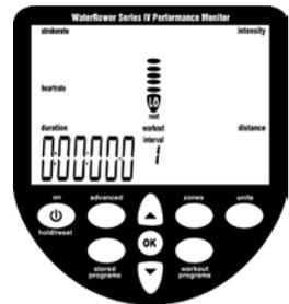
Once the first workout rest duration is reached press "OK" (the distance digits will appear along with the "distance" and distance units flags, the "workout", "interval" and "work" flags will be flashing and the zone bar will be scrolling up to HI. The number 2 will appear in the program window denominating the 2nd work session).
