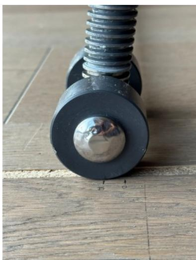
Due to the **incline mechanism** (up to 25 degrees), the **front support wheels** are slightly set in motion. The travel distance of the front rollers is between **1–2 cm** (see figure), with the wheels moving forward by about **1 cm** at maximum incline.
