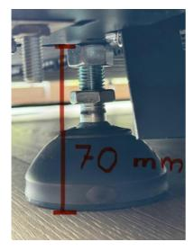
The **rear leveling feet** are fixed on the floor.
