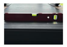
Make sure that the treadmill is aligned horizontally!
