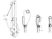
Third, shorten the recoil strap by readjusting the strap in the buckle. Be careful not to make the recoil belt too short, as the connector may catch on the forward riser.
