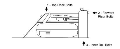
If rubbing has stopped, gently retighten the bolts in the same order. Replace the top deck cover.
