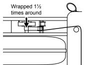
First, remove the top deck cover and check the belt alignment to make sure all straps are positioned correctly on the pulleys.
